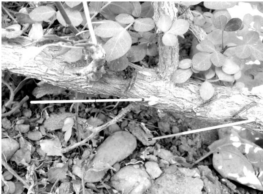
Figure 3. Insertion of capillaries into the vertical drain groove made in thick stems.
